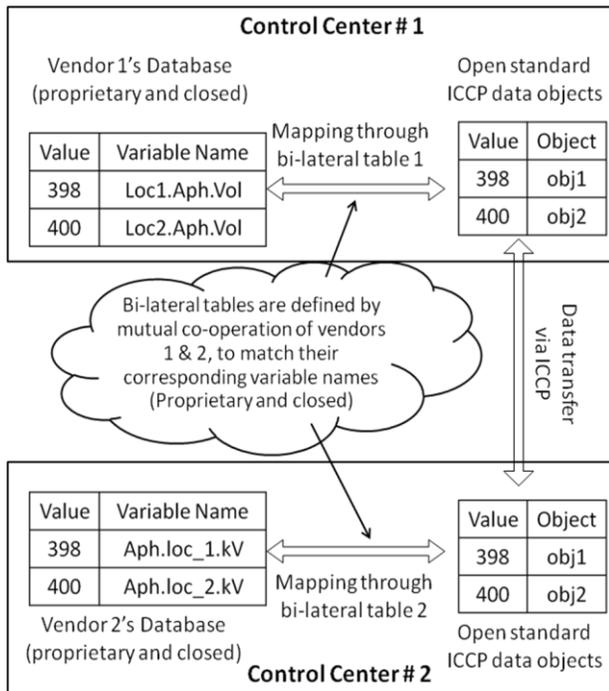
Figure 5: Typical Inter control center data transfer
