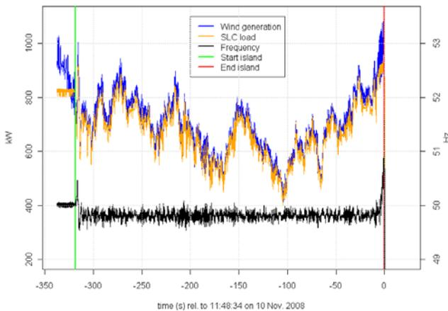
**Figure 3: Effect of the SLC During the Mini-Island Test**
