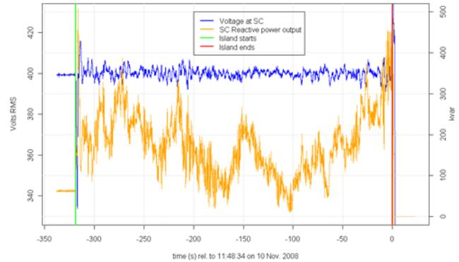
**Figure 4: Effect of the SC During the Mini-Island Test**
