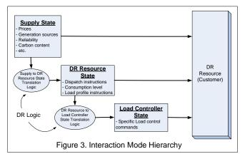
To go from Supply State (e.g. a price) to a DR Resource State (e.g. shed 100 KW) requires some sort of logic as depicted in Figure 3. Furthermore to go from DR Resource State (e.g. shed 100 KW) to specific Load Controller States (e.g. change set point on thermostat) requires another set of logic.
