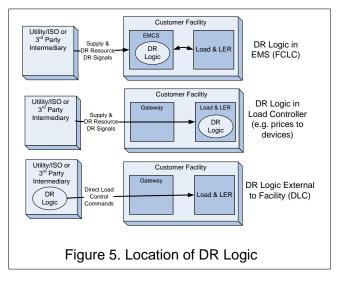
In the top scenario of Figure 5 the DR Logic is encapsulated entirely within the facility and the clearly constitutes FCLC.
