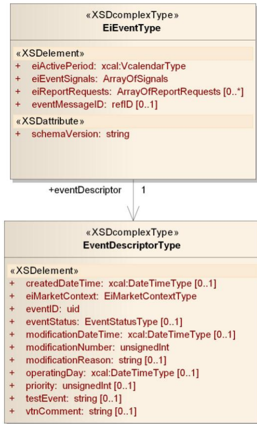
FIGURE 4 ENERGY INTEROPERATION EIEVENT AND DESCRIPTOR
