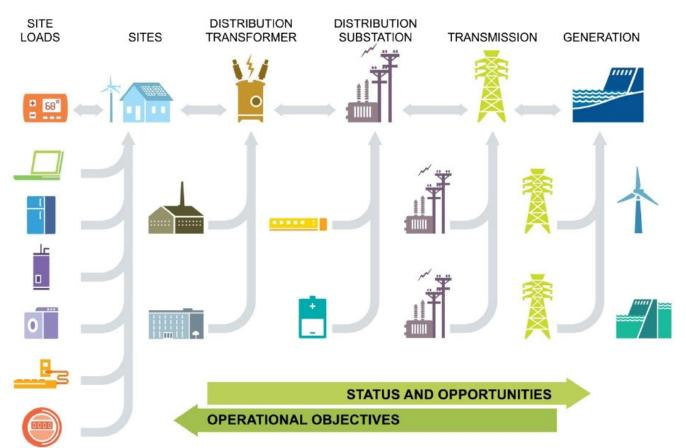
Aggregation of Power and Signals Occurs Through a Hierarchy of Interfaces
