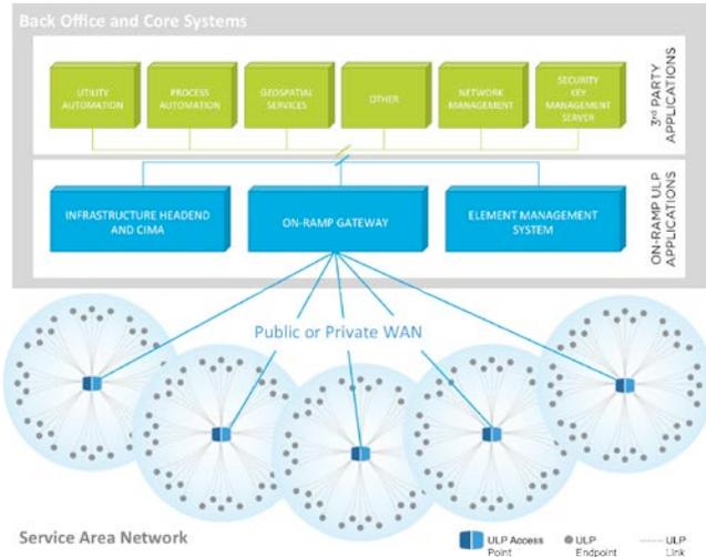
A star networking topology, on the other hand – which is relied upon by the cellular industry – features a central access point (the center of the “star”), which communicates directly with end nodes in its coverage area. End nodes, in the case of the Smart Grid, could be meters (gas, water, power), sensors, assets, etc.
